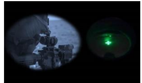
A Soldier uses the ACOG weapon sight on an M-4 weapon. The inset shows the illumination due to the presence of tritium, which facilitates pointing the target in darkness. (Stock Photos)
