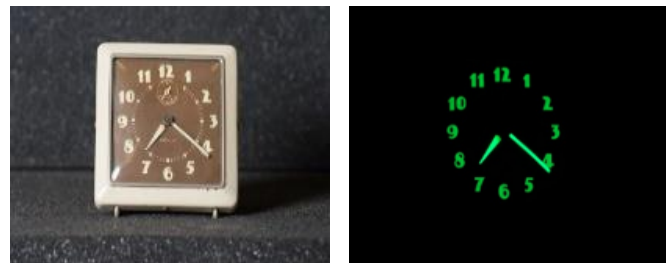
A commercially available clock with a radium-226 painted face. These pictures are under white light, and no light conditions, respectively. (Photos: APHC)
