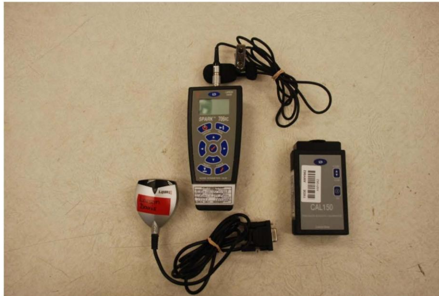
LARSON DAVIS NOISE DOSIMETER W/ CALIBRATOR AND IR UNIT MODELS SPARKS 706 AND 706RC
