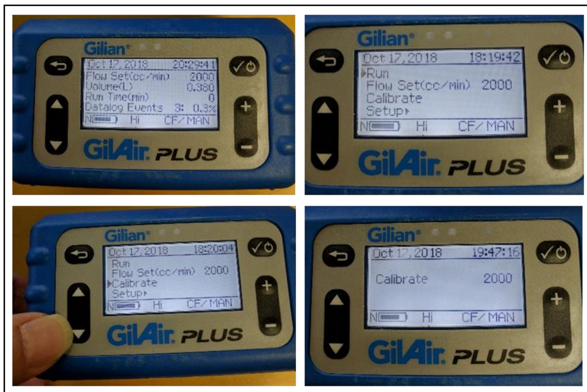
Photo 1. Gilian Pump Calibration Setup
