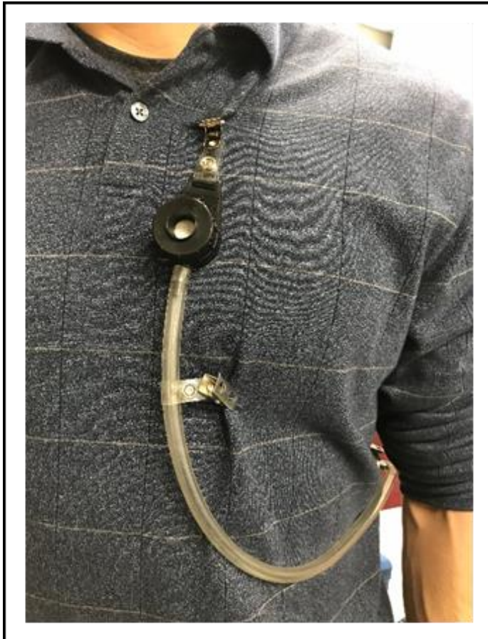
Photo 8. IOM Filter Correctly Oriented on Wearer, with Cap Removed
