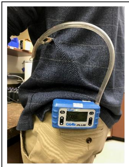
Photo 7. Gilian Pump Appropriately Attached to Belt
