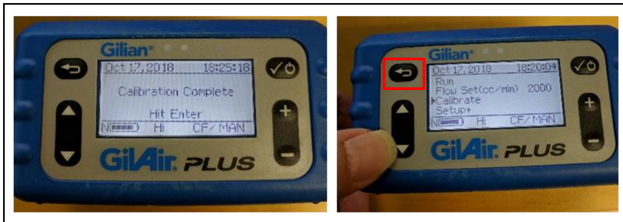
Photo 6. Exiting Out of Calibration Mode on Gilian Pump
