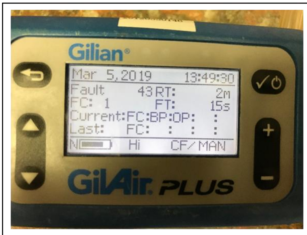
Photo 11. Fault Screen on Gilian Pump
